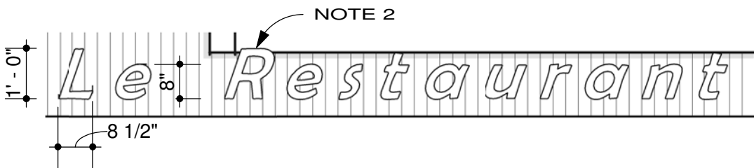
3 SIGNAGE SOUTH ELEVATION - Callout 1 3/8'' = 1'-0''
