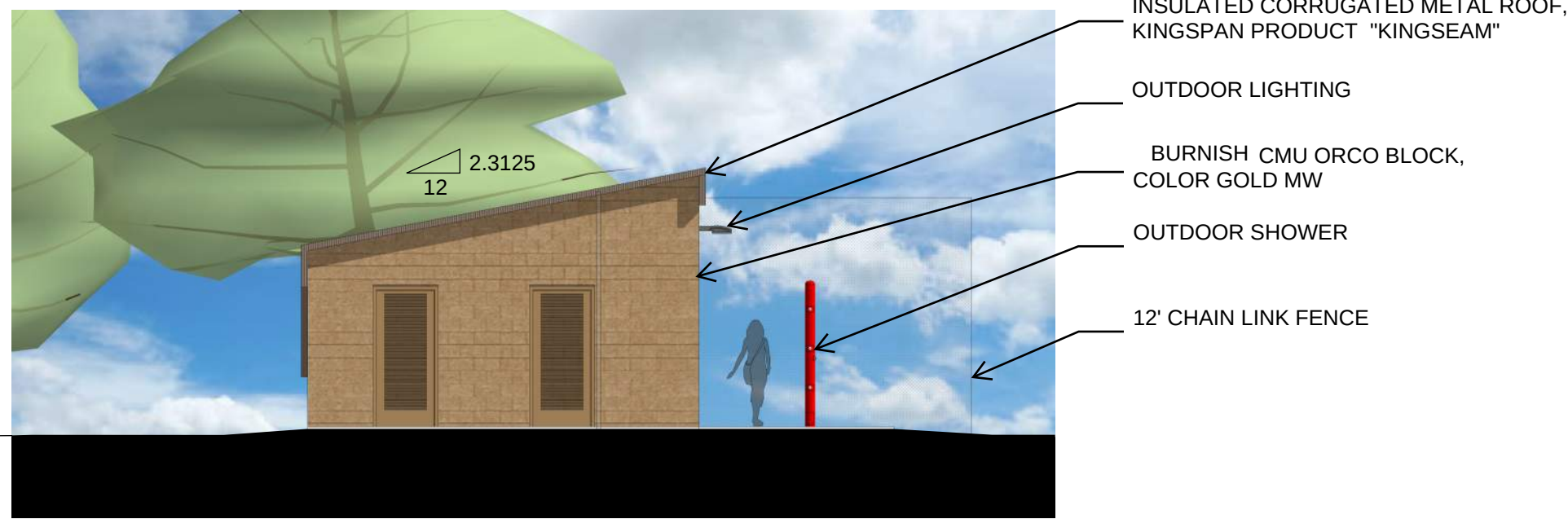
7 POOL HOUSE SOUTH ELEVATION 1/8" = 1'-0"
