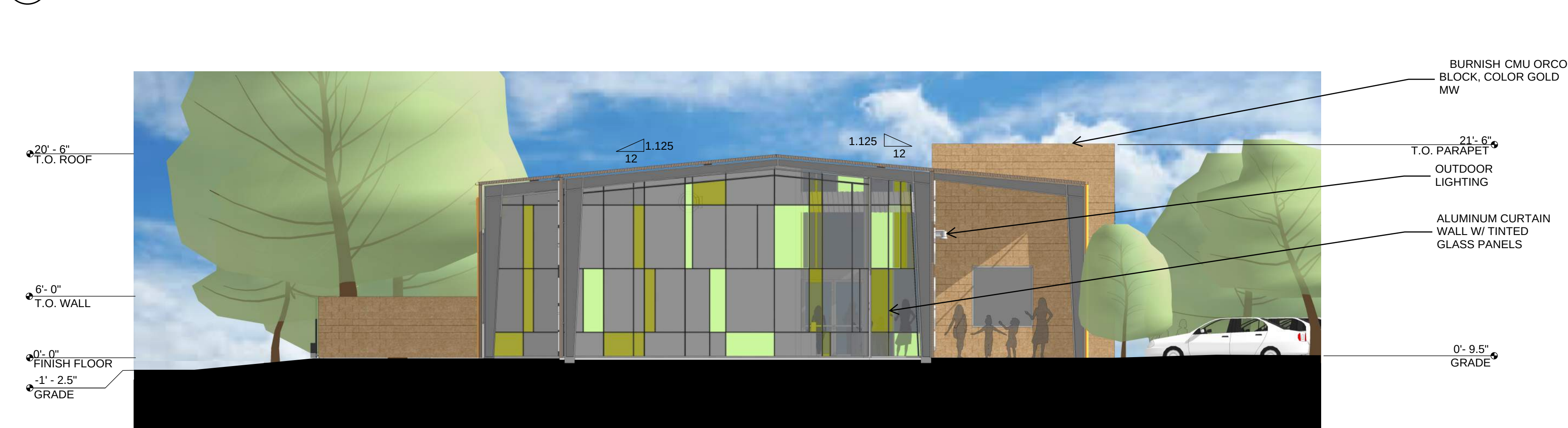
4 PROPOSED BUILDING WEST ELEVATION 1/8" = 1'-0"
