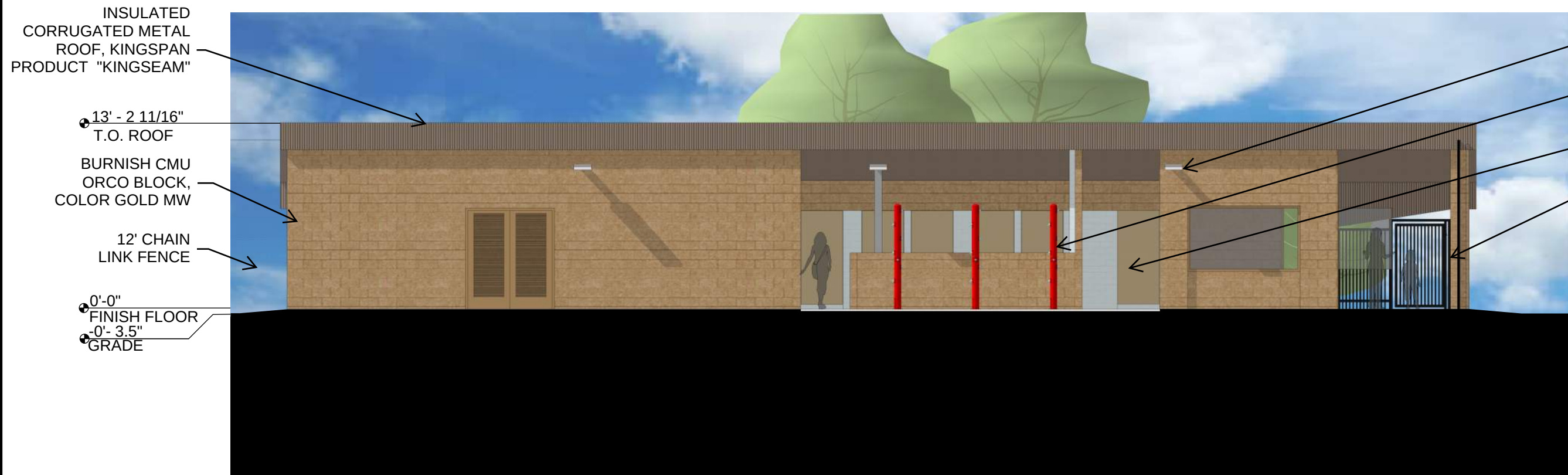
8 POOL HOUSE EAST ELEVATION 1/8" = 1'-0"
