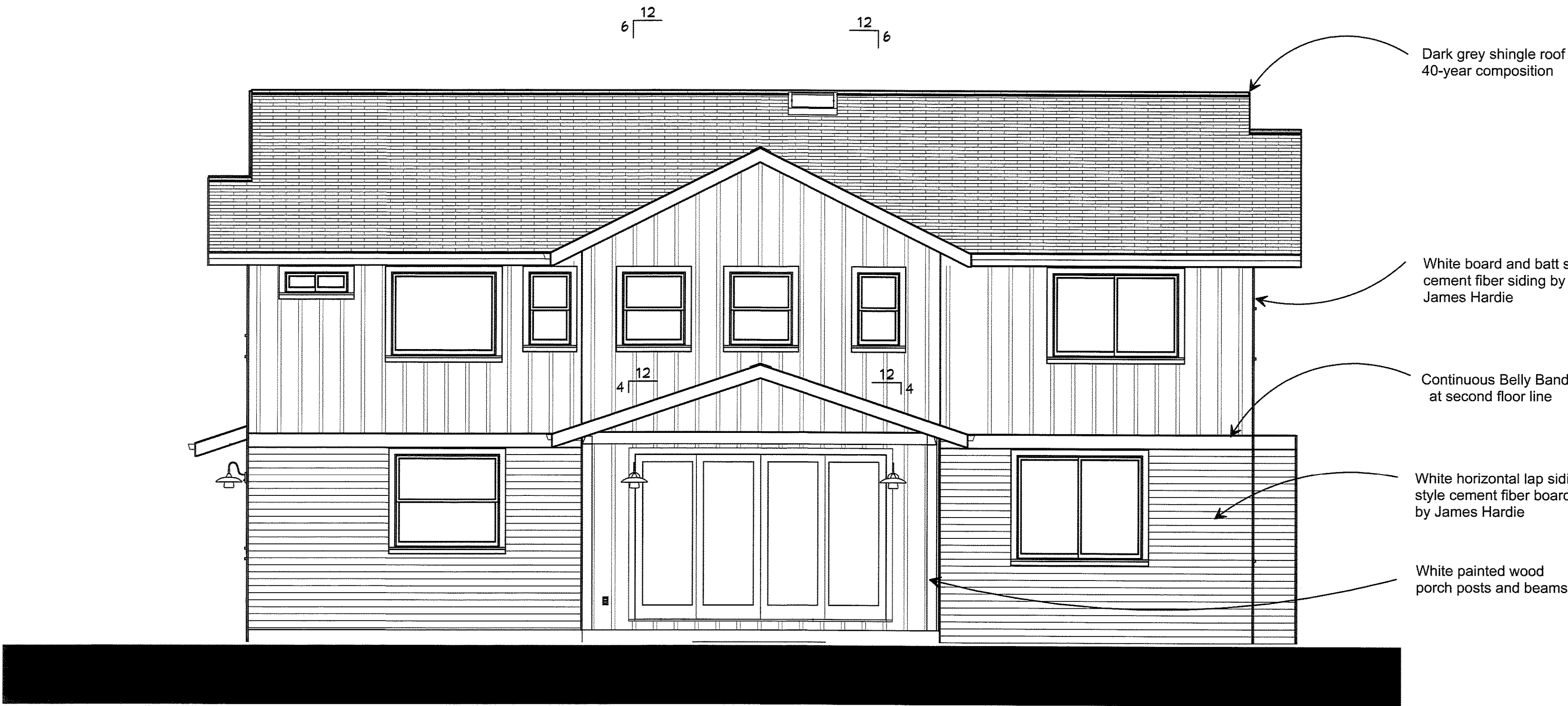
B South Elevation, Rear 1/4" = 1'-0"
