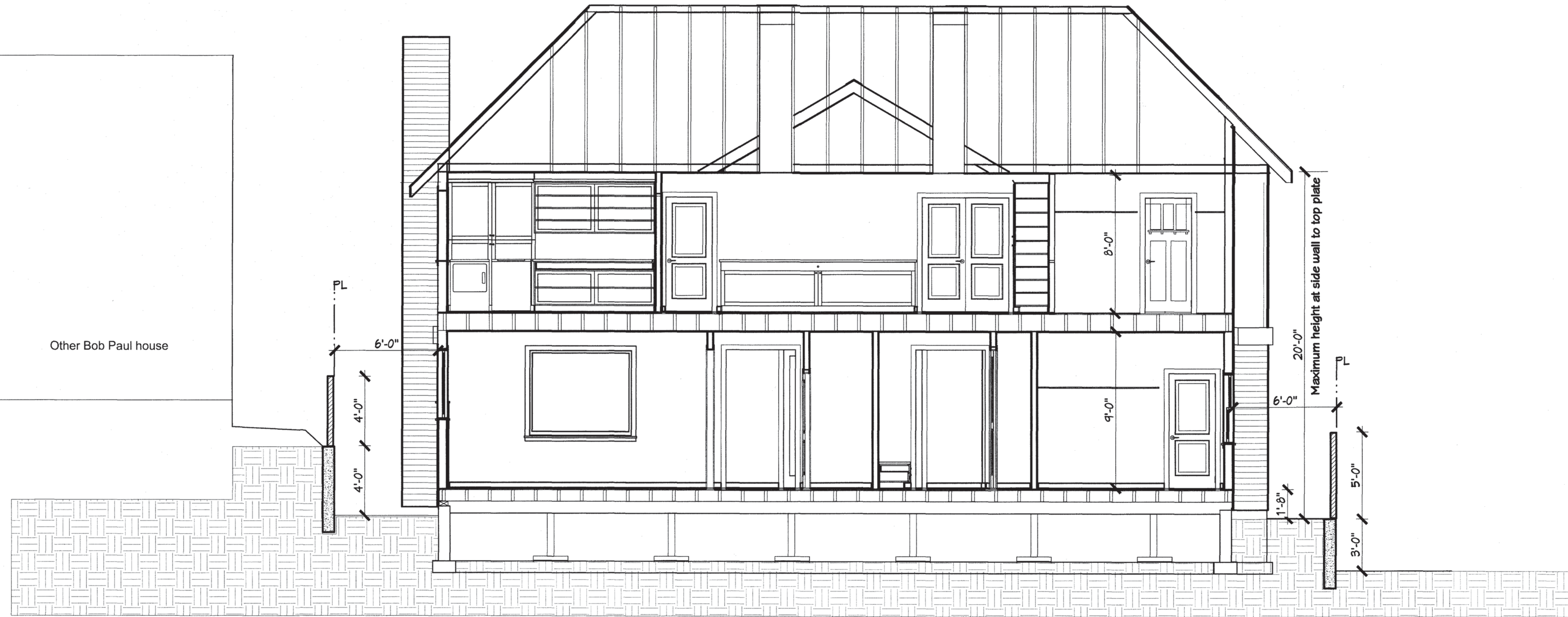
Transverse Building Section, at main ridge looking South
