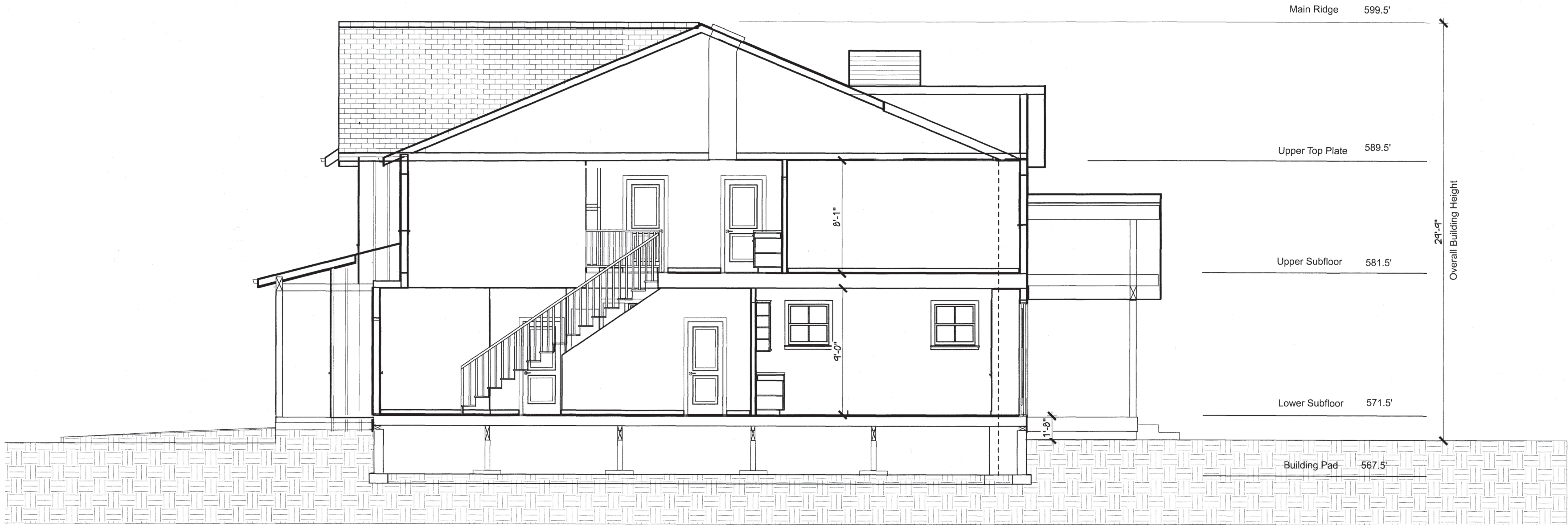
Longitudinal Building Section, at centerline of rear ridge looking East
