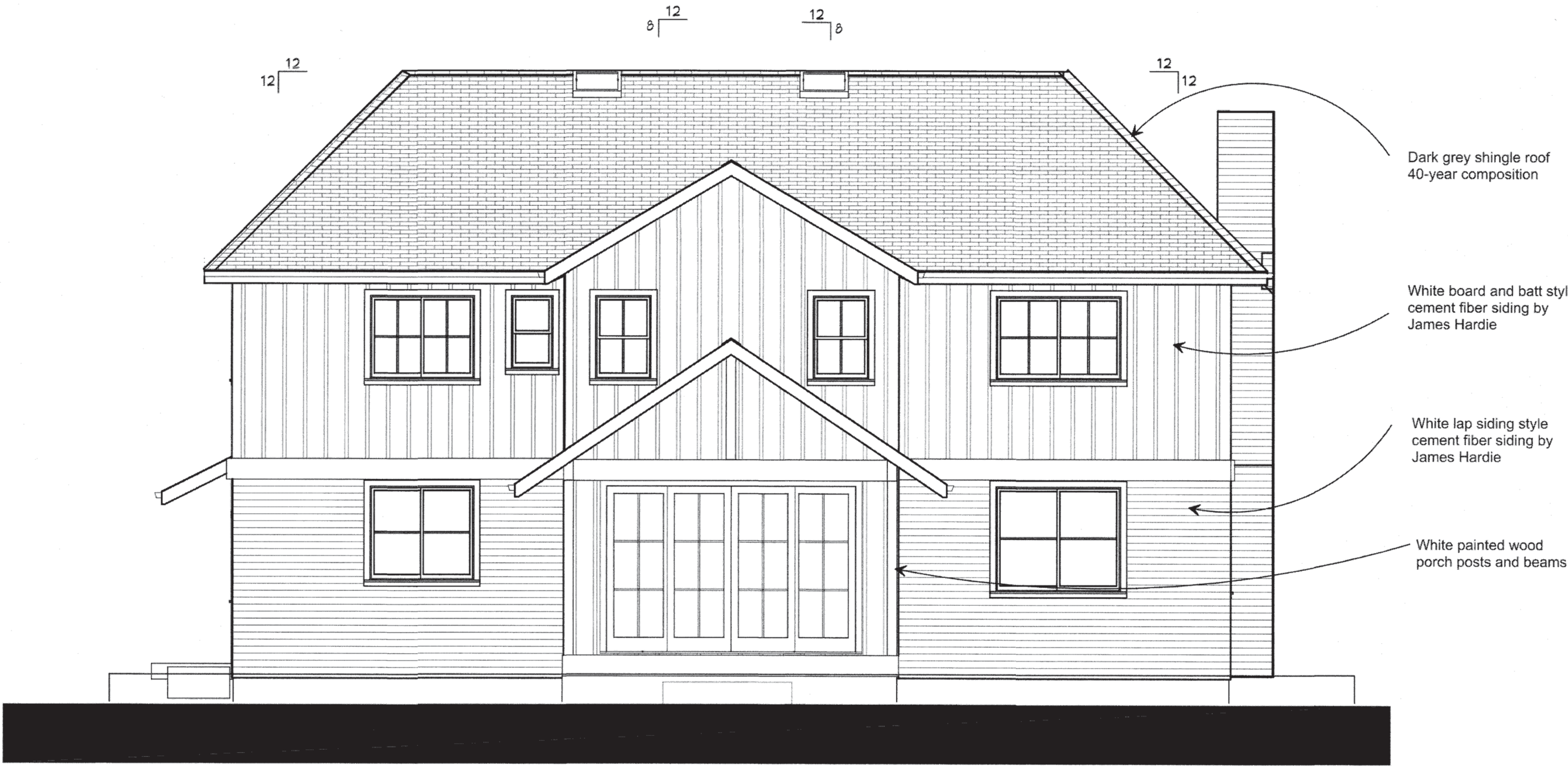
B South Elevation, Rear 1/4" = 1'-0"
